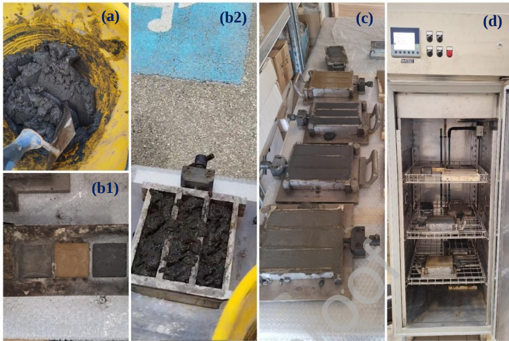
Fig. 5. Production process of the produced mortars with/without AC_{cs} /EPCM composite (a) mixing; (b1-2) molding; (c) molded samples; (d) curing in environmental chamber
