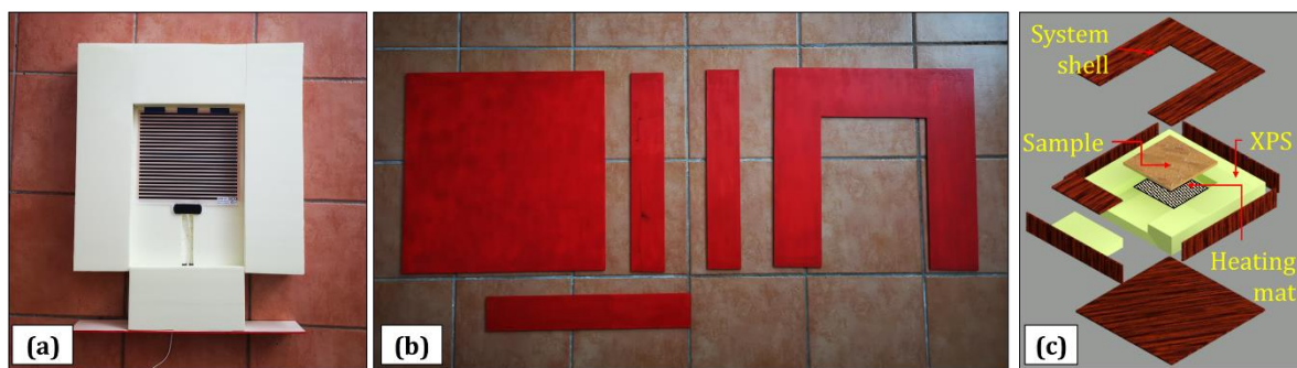
Figure 2. Internal XPS structure (a); external cladding (b); exploded view of the structure (c).
