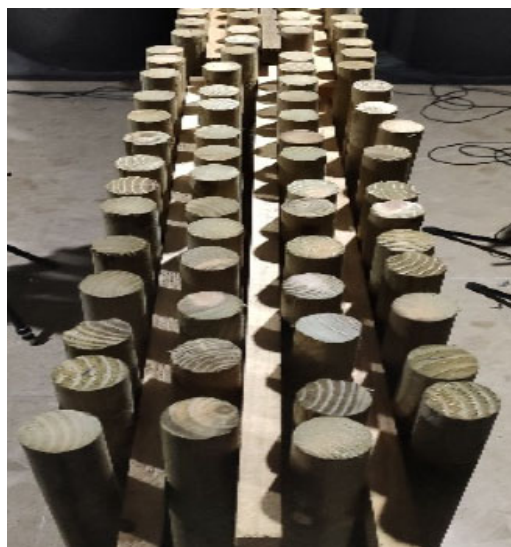
Figure 14. Example of deviations in the position of the scatterers in a wooden sonic crystal noise barrier.
